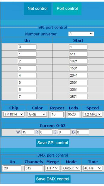
Led port refresh rate. The controller supports increased data transfer rates to the tape. All tested tapes can operate at 1 MHz, however, you must reduce the length of the data wire to 1 meter.
