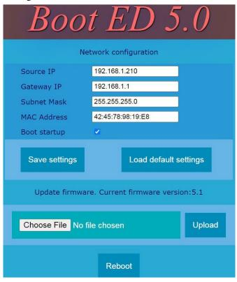
On the boot loader page, you can modify the network configuration, reset all settings to default, and update the firmware to the required version. However, in the boot loader, you can only alter the network configuration.
