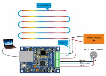
Connect to both a 5V and a 12-24V powersupply.
